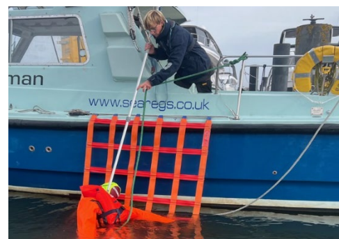
5) Once the PIW is in the cradle, the cradle can be pulled closed using the green line (in the crews left hand in the photo above)
