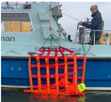
6) The purchase system can then be used to lift the PIW out of the water.
