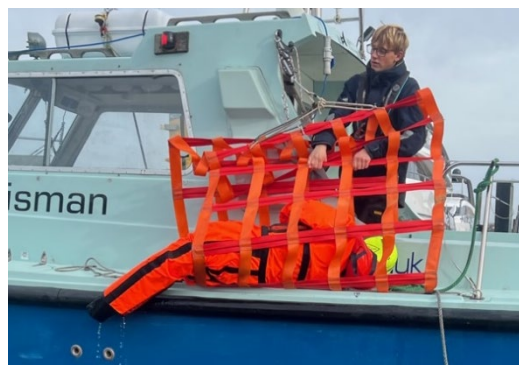
9) This process is continued until the PIW arrives at the deck edge. They are then maneuvered inboard.
