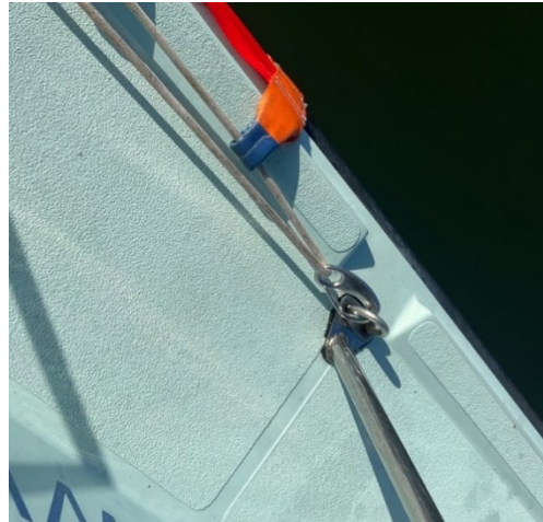
2) Carabiner clips to the U-Bolt on the deck, just aft of the access gateway.
