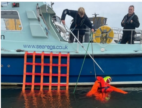
4) The cradle is then lowered into the water. Using the boat hook, the PIW can then be maneuvered into the cradle gently.
