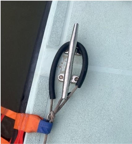
1) "Black Piped" Bowline goes round the midships cleats.
